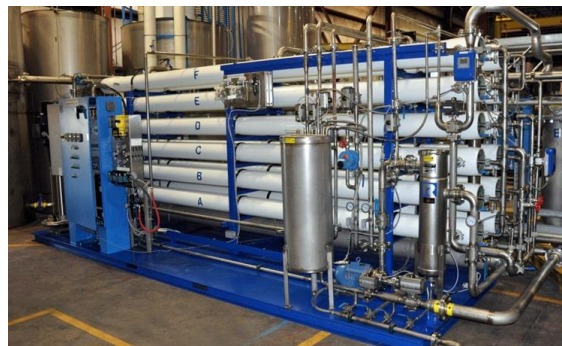
Fig 1 Water Treatment by NF Nano Filtration Method
